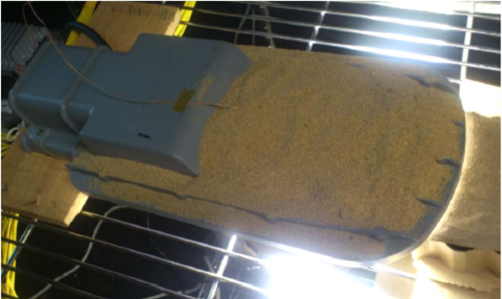
Thermal testing is also done by covering the luminaire thermal fins
